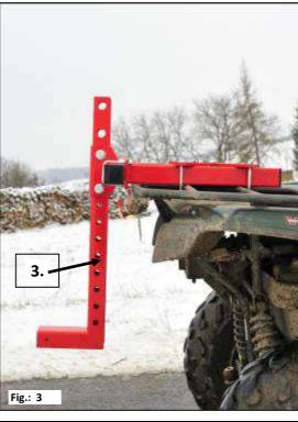
The holes on the fastening frame (fig.: 3) can be used to select the fitting surface height (fig.: 4 & 5).
