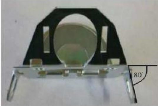
Figure 51: Bending the lateral dispersion plates
