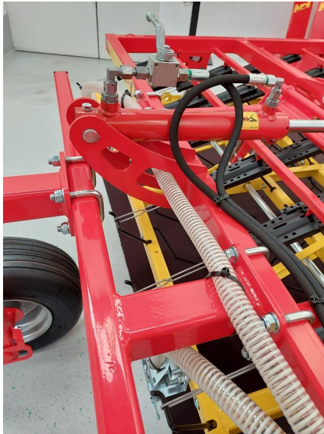
Figure 80: Hose laying along the harrow 7
