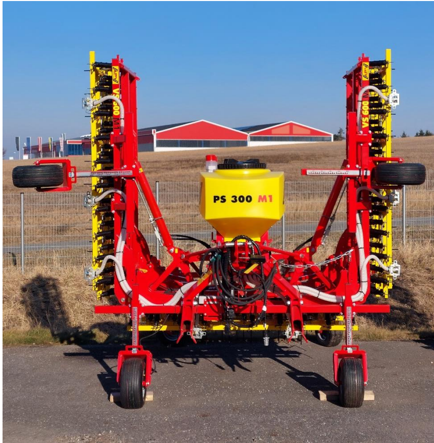
Figure 85: VS600 with PS in folded state
