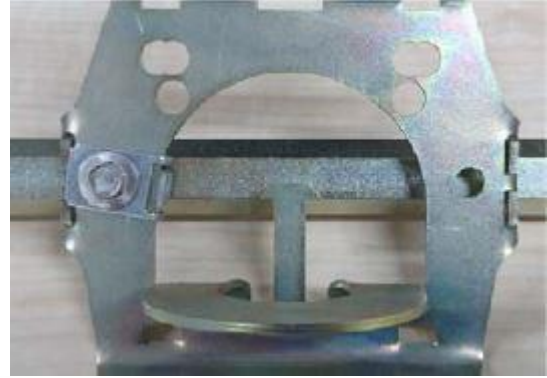
Figure 52: Dispersion plate threaded and fixed on the hexagonal bar
