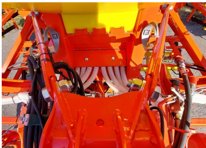
Figure 71: Hose laying starting from the PS outwards 2
