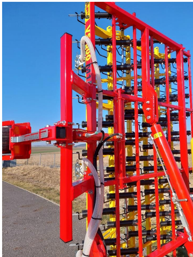
Figure 81: Hose laying along the harrow 8
