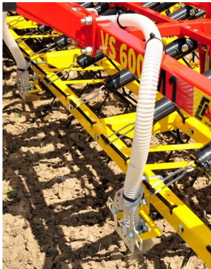
Figure 83: Hose laying along the harrow 10
