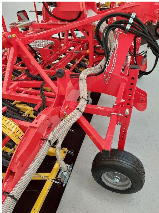
Figure 75: Hose laying along the harrow 2
