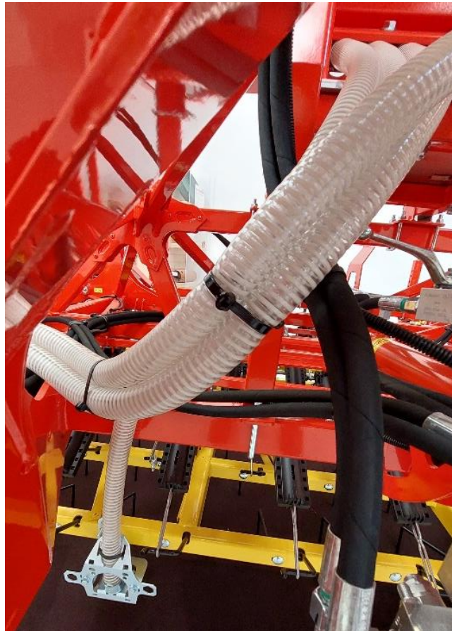
Figure 72: Hoses to the dispersion plates on centre frame 1
