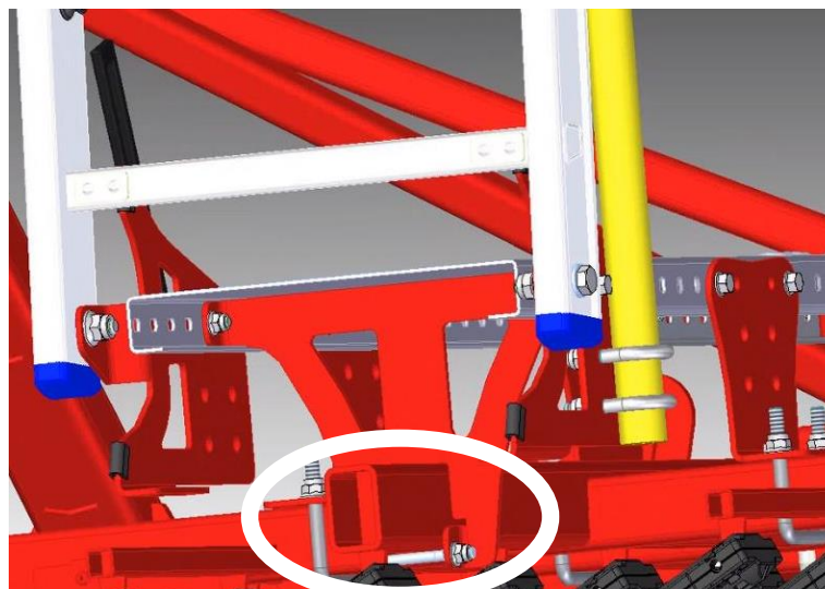
Figure 27: Fixing the platform with the screws on the hollow profile
