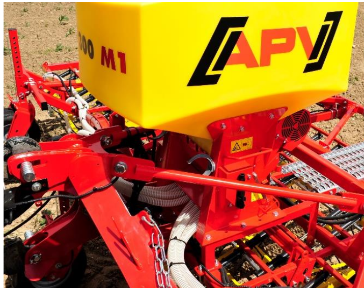
Figure 70: Hose laying starting from the PS outwards 1
