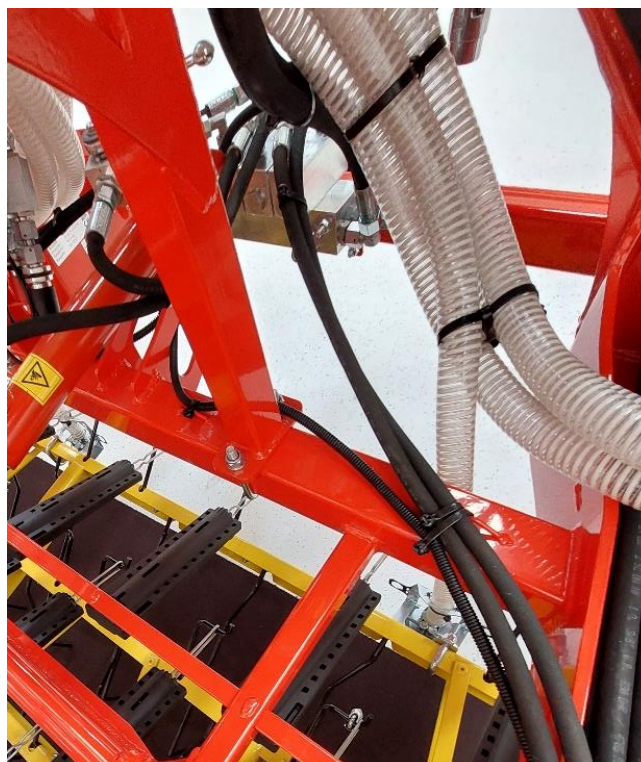
Figure 73: Hoses to the dispersion plates on centre frame 2
