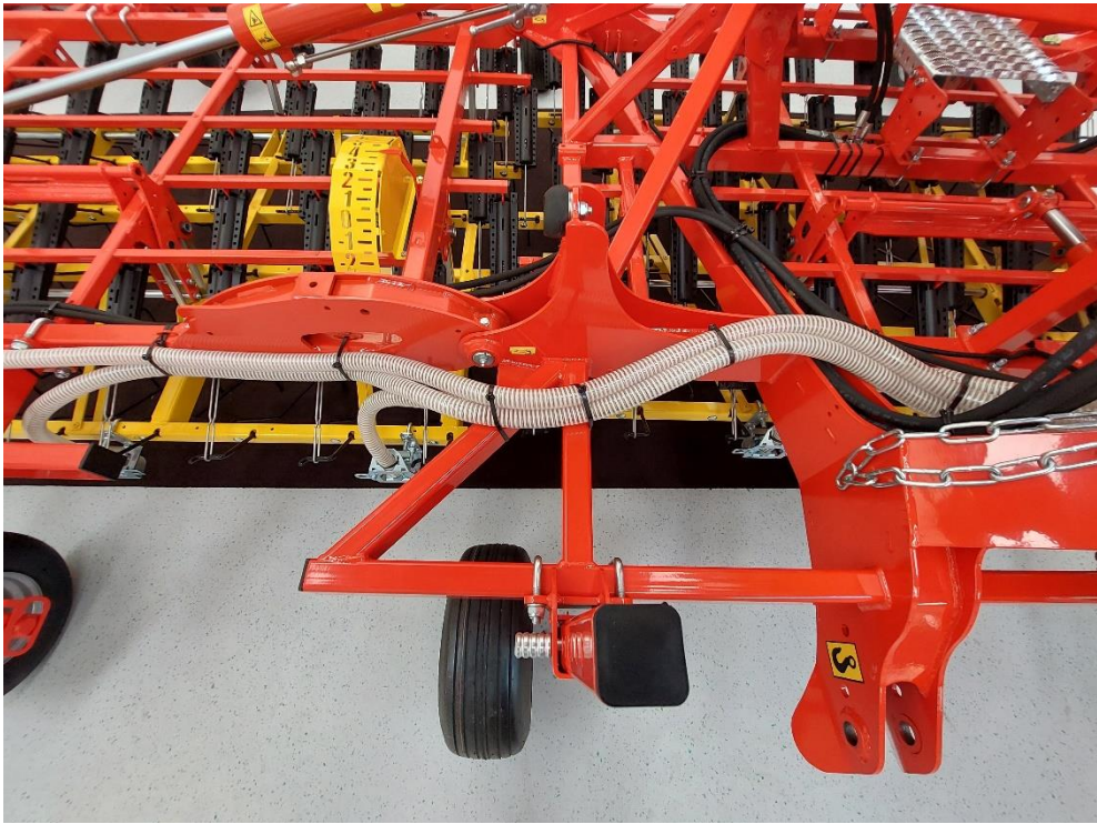
Figure 76: Hose laying along the harrow 3
