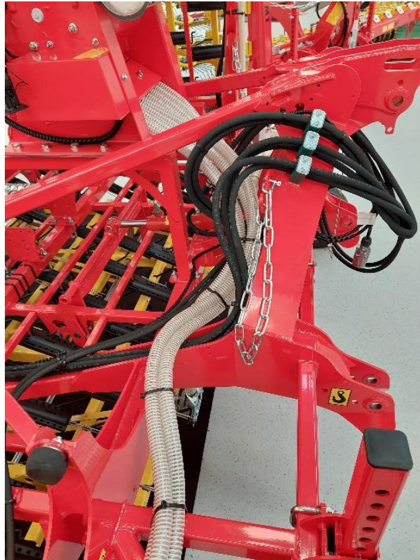
Figure 74: Hose laying along the harrow 1
