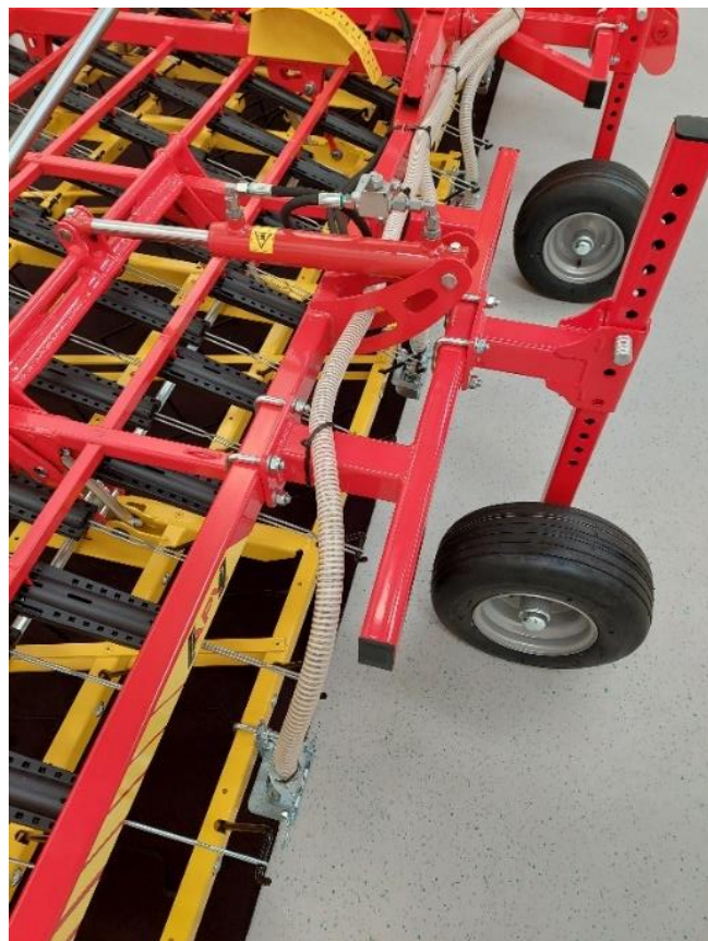
Figure 79: Hose laying along the harrow 6
